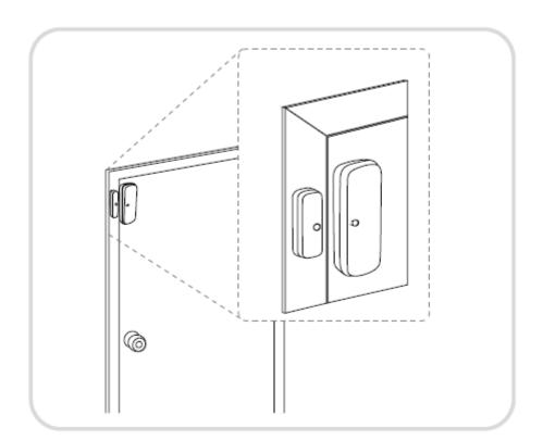
Affix your Sensor plates to a surface. The Mounting plates can be affixed using screws or double-sided tape. If you are using screws, attach both mounting plates to the respective surface using the two 20mm screws provided.
